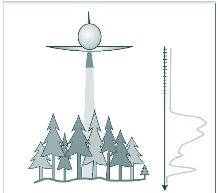
**Figure 8.** Scientists can calculate the height of trees based on the time it takes a light beam to travel from the ICESat satellite to Earth and back to the satellite. Scientists can do this because they know how fast light travels. The speed of light is 186,282 miles per second.
