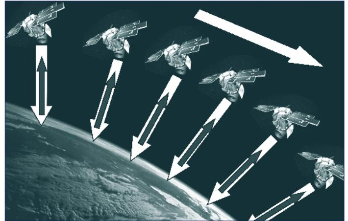
**Figure 7.** As ICESat orbits Earth, GLAS sends beams of light to Earth's surface. ICESat travels at 16,000 miles per hour and 370 miles above Earth.
